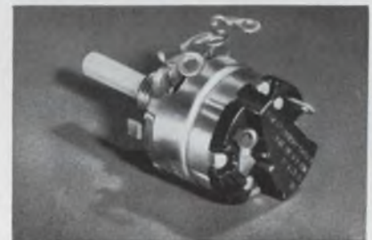
OCB breaker switch attached to volume control.
