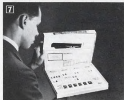
TI Designer's Kit for integrated circuits. Three different kits are offered by TI distributors.
