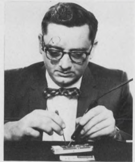
Parametric multiplier circuit in miniature S-band transmitter is tuned by Dick Moss, engineer at Sylvania Electronic Systems Div.
