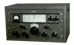
Circuitry: Transformer-powered superhet, ham bands only. Double conversion. One r.f. stage; two mixers; three i.f. stages; bandspread; "S" meter; crystal filter; BFO; noise-limiter; speaker separate. *Tube complement:* 6AK5 r.f. amplifier; 6SA7 1st mixer; 6SK7 1st i.f. amplifier; 6L7 2nd mixer; 6AK5 crystal oscillator; 6SG7 (2) 2nd and 3rd i.f. amplifiers; 6H6 detector/limiter; 6SJ7 BFO; 6SJ7 1st audio; 6V6 audio output; 6SJ7 VFO, 5Y3 rectifier.
