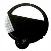
A computer-generated number strip was created as a template for replacing wiped-off numbers on the dial window (see text) with properly-sized dry-transfer numbers selected from a hobby-shop sheet (corner seen at left).
