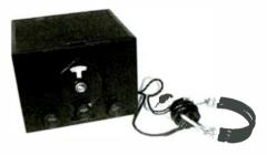
Circuitry: One r.f. stage; regenerative detector; one stage of audio; headphone operation only. Original Tube complement: for battery operation 36 r.f. amplifier; 36 detector; 37 audio output for a.c. or a.c./battery operation 35 r.f. amplifier; 35 detector; 27 audio output.
