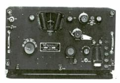
Circuitry: Dynamotor-powered (BC-312) or transformer-powered (BC-342) superhet. Two r.f stages; two i.f. stages; crystal filter (some models); BFO; speaker separate. *Tube complement*: 6K7 (2) 1st and 2nd r.f. amplifiers; 6L7 mixer; 6C5 oscillator; 6K7 (2)1st and 2nd i.f. amplifiers; 6C5 BFO; 6R7 detector/1st audio; 6F6 (audio output).
