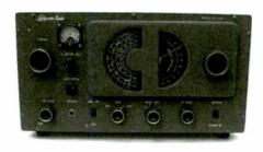
Circuitry: Transformer-powered superhet. One r.f. stage; two i.f. stages; bandspread; Smeter; BFO; noise-limiter; speaker separate. *Tube complement:* 6BD6 r.f. amplifier; 6BE6 oscillator/mixer; 6BD6 (2) 1st and 2nd i.f. amplifiers; 6AV6 detector/AVC/1st audio; 6AV6 BFO/limiter; 6AR5 audio output; 5Y3 rectifier.
