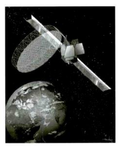
Thuraya phones transmit up to the satellite between 1626.5 and 1660.5 MHz and receive from the satellite between 1525.0 to 1559.0 MHz.
