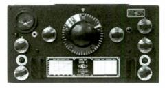
Circuitry: Features and tube lineup varied over the years. Model illustrated has two r.f. stages; two i.f. stages; separate mixer and local oscillator; crystal filter; combined detector and AVC stage; first audio amplifier; noise limiter; audio output stage; CW oscillator; "S" meter. Requires separate power supply and speaker.
