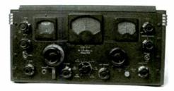
Circuitry: Transformer-powered superhet. Two r.f. stages; two i.f. stages; push-pull audio output; bandspread; "s" meter. crystal filter; BFO; noise-limiter; speaker separate. *Tube complement:* 6SK7 (2) 1st and 2nd r.f. amplifiers; 6SA7 mixer; 6SA7 oscillator; 6L7 1st i.f. amplifier/noise limiter; 6SK7 2nd i.f. amplifier; 6B8 detector/s-meter amp., 6B8 AVC amp.; 6SK7 noise amp.; 6H6 noise rectifier; 6J5 BFO; 6SC7 first audio; 6V6 (2) audio output; 5Z3 rectifier.
