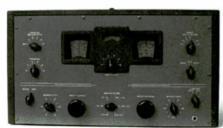
Circuitry: Transformer-powered superhet. One r.f. stage; three i.f. stages; voltage-regulated oscillator; bandspread; "s"-meter; crystal filter; BFO; noise-limiter; speaker separate. *Tube complement:* 6SS7 r.f. amplifier; 6K8 oscillator/mixer; 6SS7 (3) 1st, 2nd and 3rd i.f. amplifiers; 6H6 detector/noise limiter; 6SN7 1st audio/S-meter amplifier; 6SJ7
