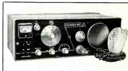
What a rig the Courier 1 was! Thirty years ago it had a triple conversion receiver in an era when other CB rigs were either super-regens or single conversion.
