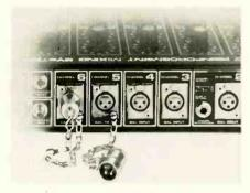
nect directly to female receptacles, shorting circuits together. This feature is said to virtually eliminate hum and noise pickup from any unterminated circuitry. A six-inch chain is provided to anchor the shorting plug,
