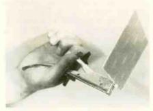
and model parts. And you can use it to trim undersized holes to fit, notch clearance on flanges of cabinets or air ducts.
