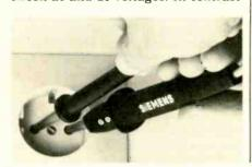
to the conventional neon testers, this new tester also indicates polarity. The new device consists of two black handles connected by a 60 cm cable. The bare test probes protrude from red plastic sleeves. One of the handles contains a ceramic PTC resistor, which is connected in series with two antiparallel LEDs and very rapidly reduces a test current to a tolerable value at any voltage. Priced at \$14.90.
