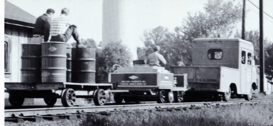
(Above) Hi-lo rail car tows spray rig and conventional push car with empty steel drums to source of water supply in preparation for trial run on May 22, last. (Right) Sprayer functions perfectly under watchful eyes of Ed Lacko (l) and Ralph Kauffman (r).
