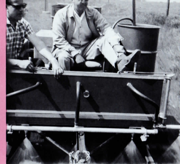
(Above) Hi-lo rail car tows spray rig and conventional push car with empty steel drums to source of water supply in preparation for trial run on May 22, last. (Right) Sprayer functions perfectly under watchful eyes of Ed Lacko (l) and Ralph Kauffman (r).
