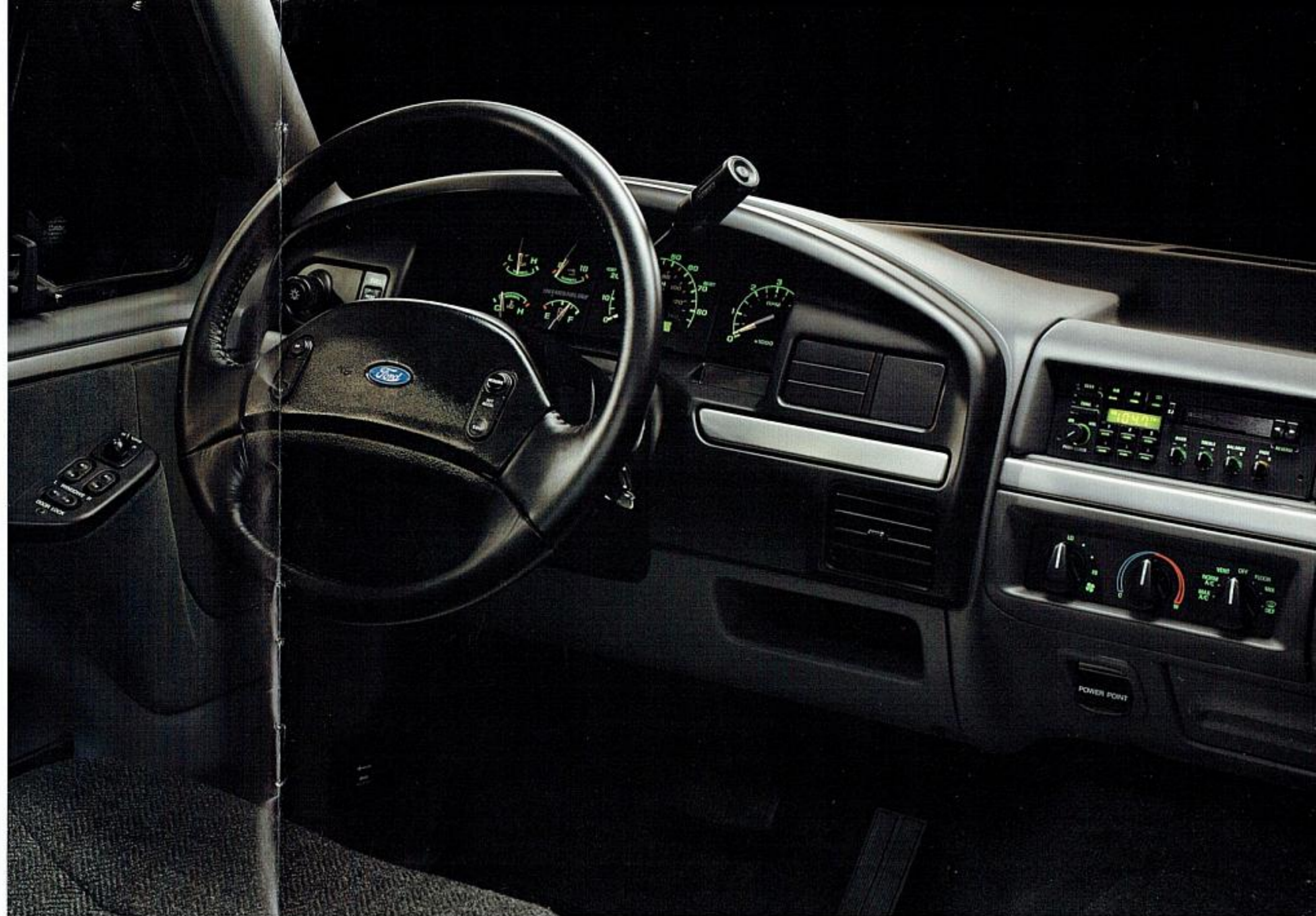
The F-Series interior has been redesigned for 1992—giving it a more contemporary appearance. The XLT Lariat is pictured above in Dark Charcoal. Yet, we've kept the things that have proven popular over the years: full instrumentation, including oil pressure and temperature gauges, voltmeter, optional tachometer; plus pivoting vent windows. Some equipment shown on these pages may be optional.
