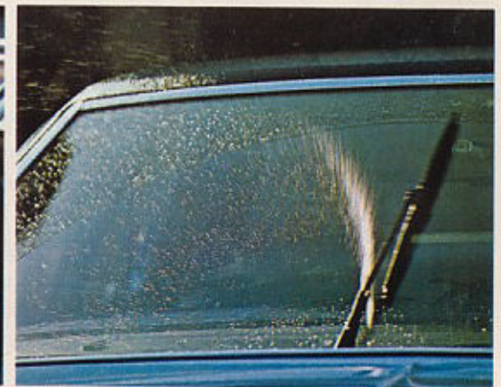
Wiper-mounted washer jets
