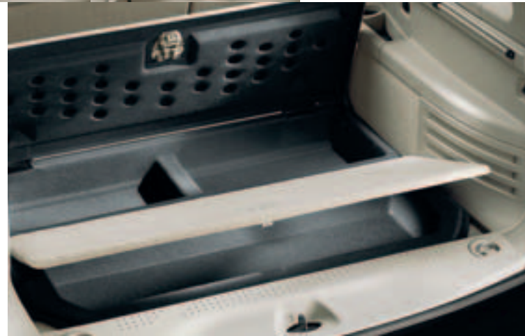
The cargo management system's middle and rear compartments open towards the rear. A removable organizer helps to keep small items in place.
