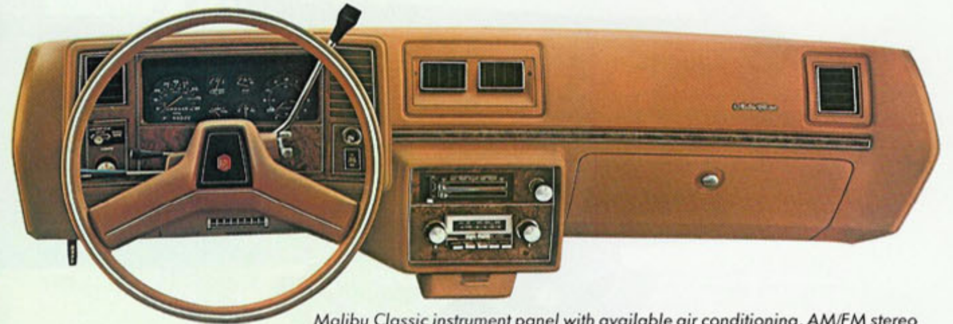
Malibu Classic instrument panel with available air conditioning, AM/FM stereo radio, rear window defogger control, intermittent windshield wiper system, Gage Package, twin remote Sport mirrors and automatic speed control.
