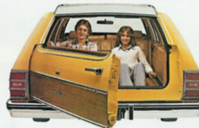
Your Chevrolet Caprice Classic or Impala Station Wagon features a three-way doorgate that swings wide to let people enter the available rear-facing third seat. Or a quick turn of the key and you can lower the glass for easy access to the rear. The door will open sideways with the glass up or down.
