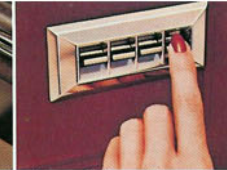
Power windows. Raise and lower your wagon's windows from a master control panel.
