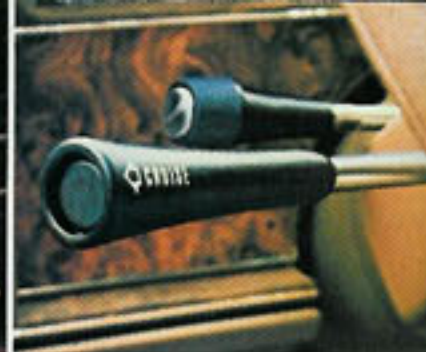
Automatic speed control. Maintains your set speed until the brake pedal is touched.
