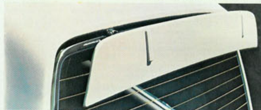
Rear window air deflector. Helps keep snow, dust and moisture from accumulating on the rear window. Included with available roof carrier on full-size wagons.
