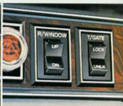
Power tailgate lock. Lock or unlock the tailgate from inside wagon. (Full-size wagon only.)
