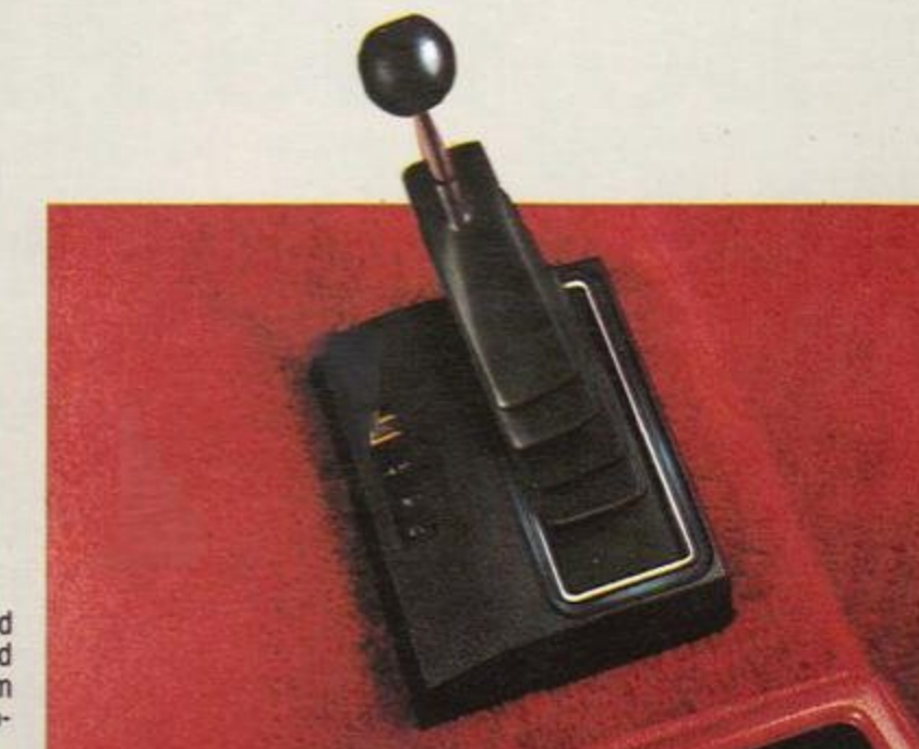
4-WD transfer case is controlled through this shift lever. Synchronized gearing permits you to shift from 2-wheel to 4-wheel drive without stopping at speeds under 25 MPH.
