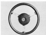
Custom Sport Steering Wheel (Code 462—UPC N31). A new, shallow-dish design, with large padded center and soft, simulated leather outer rim. Spokes are brushed stainless steel. Black only. Standard on Grand Am. Available on Grand Prix. (F)
