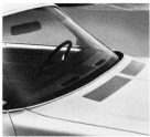
Concealed Windshield Wipers (Code 432—UPC 036). Completely concealed. Dual-speed and parallel-action wipers, with articulating left wiper for superb visibility. Available on Firebird and Formula. Not available on Ventura or Ventura Custom. Standard on all other models. (F)
