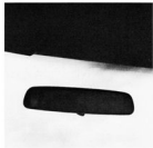
The Console Windshield Antenna is standard equipment on all Pontiacs, except Ventura and Ventura Custom, even when a model is not factory-equipped with a radio. An outside antenna need not be installed if a radio is added later. Ventura and Ventura Custom get a Windshield Antenna only when a factory-installed radio or Soft-Ray glass is ordered.
