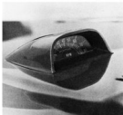
Hood-mounted Tachometer. Right out in front of the windshield, on the driver's side, for easy, instant read-out. Available with V-8 engines on Firebird, Esprit, Formula (Trans Am standard equipment includes instrument panel tachometer). (F)
