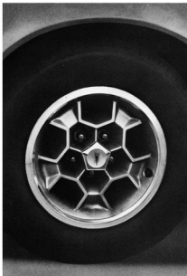
Honeycomb Wheels (Code 478—UPC PD5). A Pontiac exclusive, the deep-set "honeycomb" design gives the look of rugged cast metal. The honeycomb face is made of Goodyear Neothane ® , bonded to a steel disc that is welded to the wheel rim. Neothane is highly resistant to ricking and scratching and is unaffected by salt, road tar and other chemicals which normally attack most metal wheels. Includes trim rings. Available on Firebird, Esprit, Formula, Trans Am, LeMans, LeMans Safari, LeMans Sport Coupe, Grand Am and Grand Prix. (F)*
