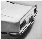
Rear Air Spoiler (Code 632—UPC D86). Spoiler—a three-piece, rear-deck attachment—adds the sporty Trans Am look to either the Firebird or Formula. Not available with Esprit. (F)
