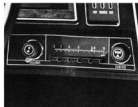
AM Radio (Code 411-UPC US8). Included in basic group. Available on all models. Completely transistorized. Five pushbuttons and tone control. (F,D)
