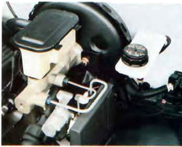
Rear wheel anti-lock brake control unit
