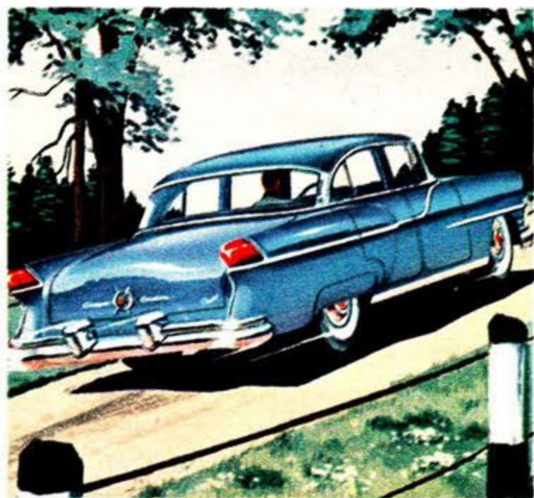
Steep grades, like this 35% rise in the Proving Grounds, are a real test of power and transmission—a place, too, to make sure of the holding power and safety of the brakes.
