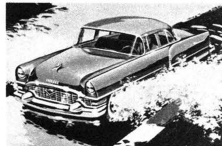
Big splash! In the thousands of miles of rigorous testing the new Packard was forced to undergo, test cars were thoroughly drenched in water trough to check body sealing, engine and chassis operation in simulated flood conditions.
