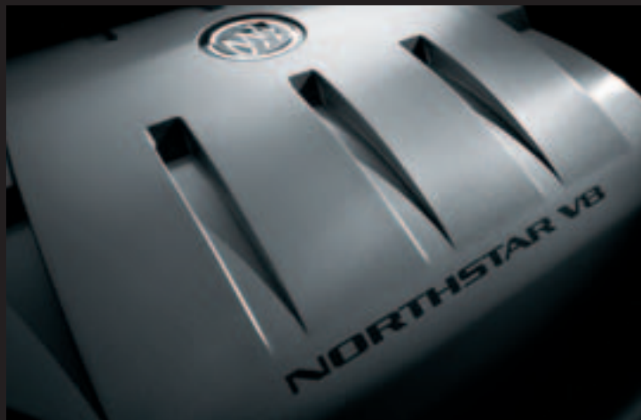
The 4.6L Northstar V8 engine produces 275 hp at 5600 rpm, and 292 lb.-ft. of torque at 4000 rpm.
