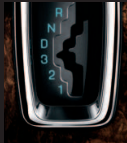
Lucerne's four-speed automatic transmission employs a gated shifter that enables you to manually select gears.
