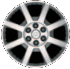
A – 17" x 6.5" steel with bolt-on wheel covers
