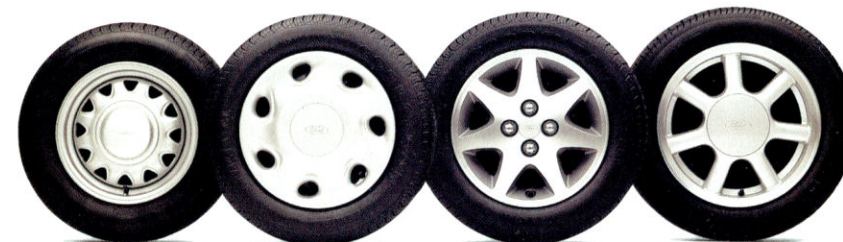
Escort wheels, left to right: standard semi-styled stamped steel wheel; LX full luxury wheel cover; seven-spoke aluminum wheel (Sport Appearance Group); GT styled aluminum wheel.
