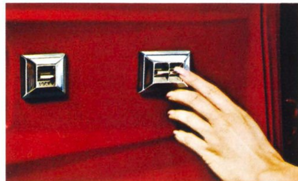
Shown left, power door lock system has a control on each door to lock or unlock both doors. Right, power windows can be adjusted by driver using master switch; separate button located on right front passenger side.
