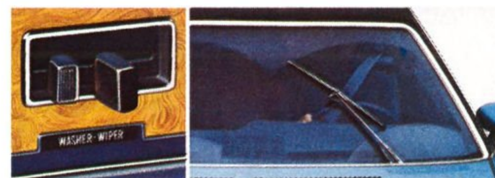
New intermittent windshield wiper system, handy during light rain or mist, lets driver select a wipe cycle with a delay of from one to 10 seconds between each wipe.
