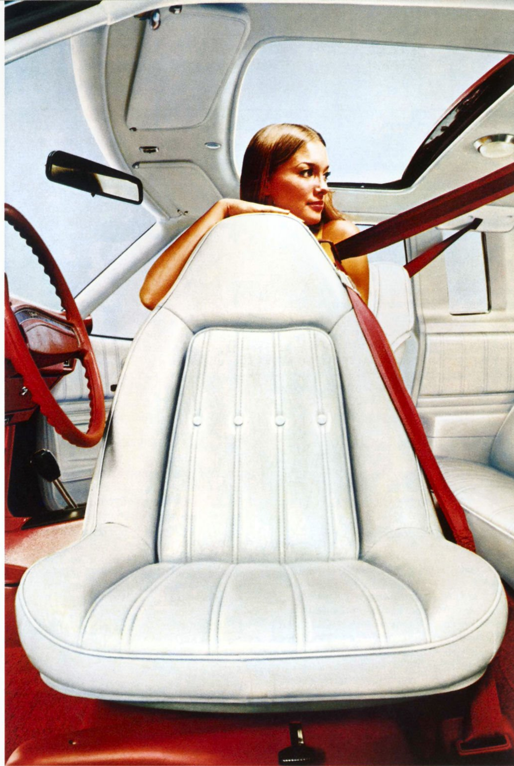
Swivel bucket seats rotate a full 90° to make getting in and out that much simpler. Shown in white vinyl with red interior accents. (See back cover for complete color selection.) Also shown above, electrically operated Sky Roof brings in the sun and outside air at the touch of a button (not available with full vinyl roof cover).
