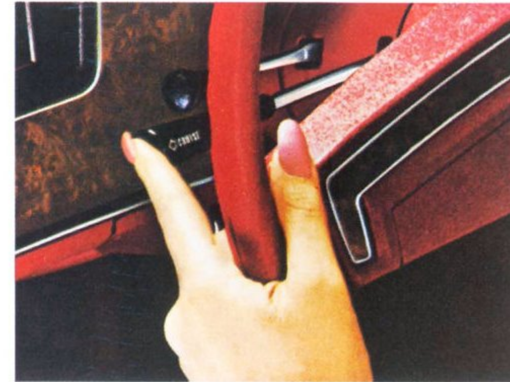
Cruise-Master speed control holds a pre-selected speed, then disengages when brake is used.
