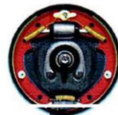
New Safety-Master Brakes —Up to 6% more durability; surer stops with 27% more bonded lining area. Wheel slots permit a flow of cooling air over drums, special flaps carry away heat.
