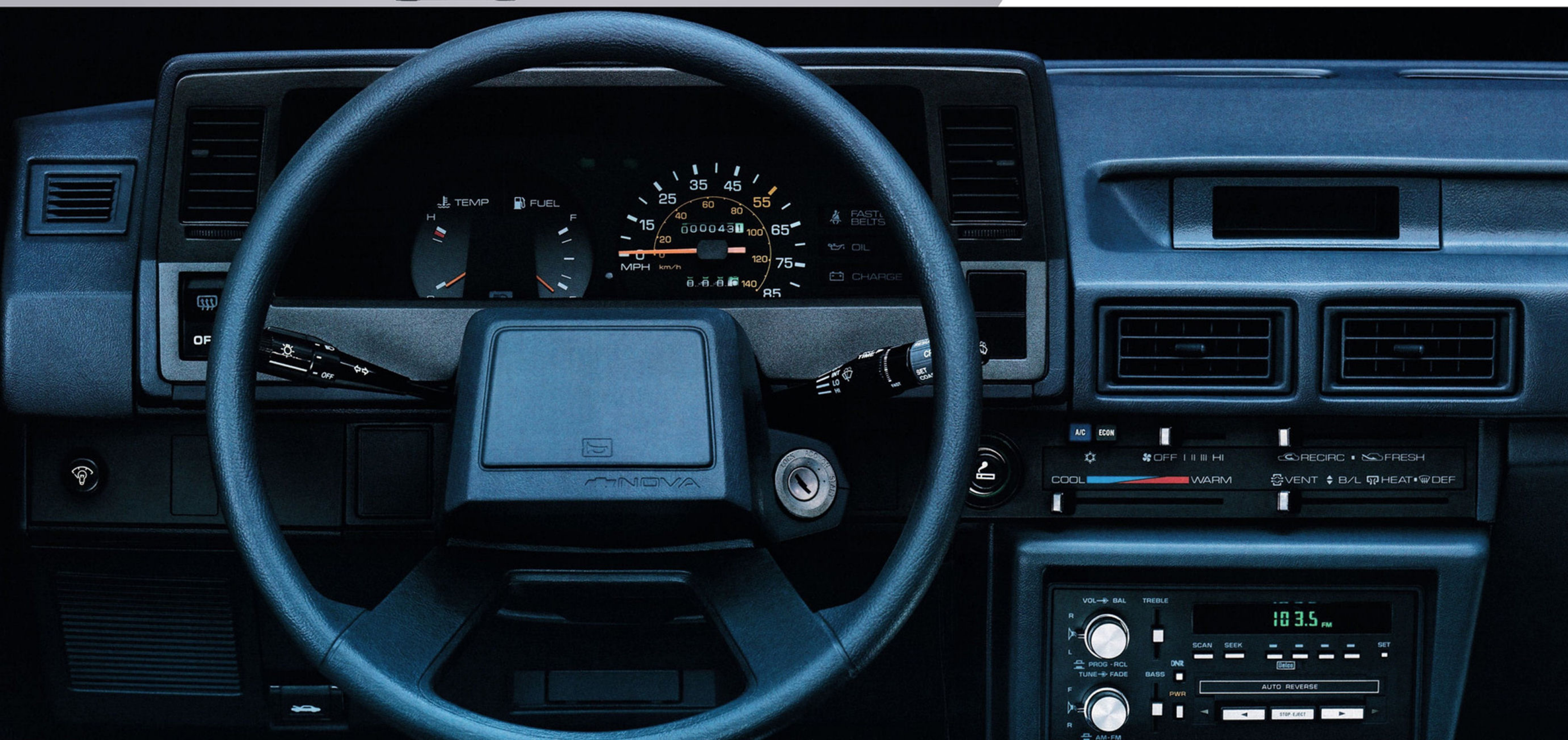
Nova CL instrument panel in Blue with optional air conditioning, Delco AM/FM stereo radio with Seek and Scan, stereo cassette tape and clock, electronic speed control and intermittent windshield wipers.
