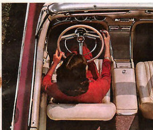
With the wheel in normal position, the selector lever can now be moved to "N" (Neutral)—the only control you need to touch to lock the wheel securely, safely.
