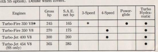
For 1971, all Monte Carlo engines have been designed to operate efficiently on the new no-lead or low-lead gasolines. In addition to the lower exhaust emissions attainable with this engine/fuel combination, there are benefits in longer life for your spark plugs, exhaust system and other engine components. If these no-lead, low-lead gasolines are not available, any leaded regular grade gasoline with a research octane number of 91 or higher may be used.
