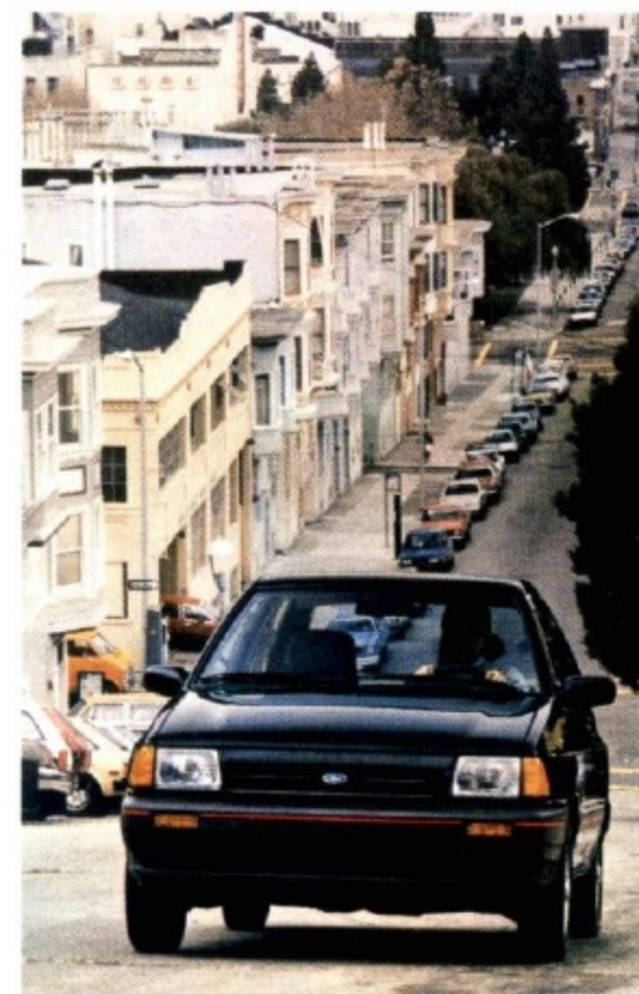
Front-wheel drive puts the combined weight of the engine and transaxle over the driving wheels, which gives Festiva good traction in adverse driving conditions.
