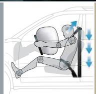
3-POINT SEAT BELTS. STANDARD FOR ALL SEATING POSITIONS IN THE SPORTAGE. THE FRONT SEAT BELTS ALSO INCLUDE PRETENSIONERS. THESE AUTOMATICALLY RESTRAIN PASSENGER MOVEMENT, IF NECESSARY, AND WORK IN CONJUNCTION WITH A LOAD LIMITER, WHICH HELPS TO REDUCE SECONDARY INJURY BY SENSING AND ADJUSTING EXCESS
