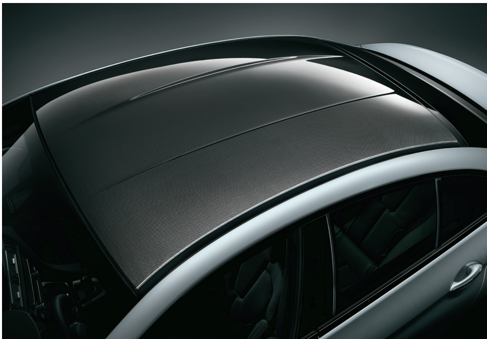
Carbon-fibre roof with aerodynamic contouring.
