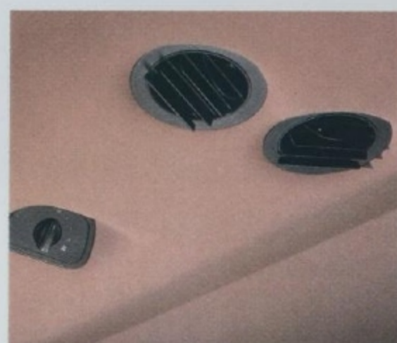
The new high-capacity air conditioning option is 50% improved in rear compartment circulation. Includes rear controls.
