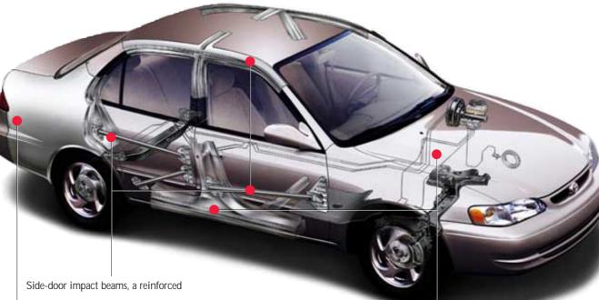
Side-door impact beams, a reinforced passenger compartment and energyabsorbing trim inside help ensure occupant safety.
