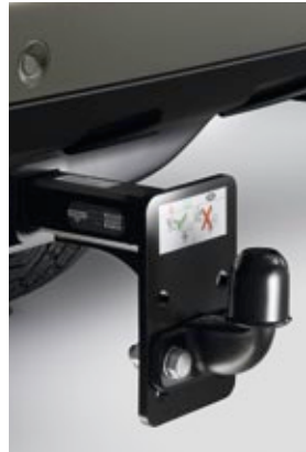
Multi-Height Tow Bar** VUB000720 Offers three different towing height options. Lowest tow ball position 360mm from ground. 3,500kg trailer load capacity (150kg trailer nose load).
