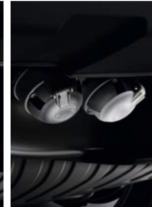
12N/12S Type Towing Electrics† VPLMT0006 Provides all trailer rear lighting and interior equipment power, where required. Supplied as a combined kit. 2010 Model Year vehicles onwards.
