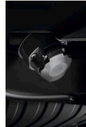
13 Pin Type Towing Electrics† VPLMT0007 European style towing electrics, capable of supplying all trailer rear lighting and interior equipment power. 2010 Model Year vehicles onwards.
