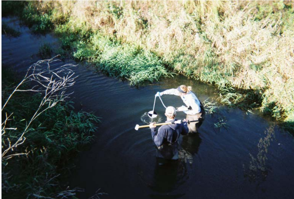
Photograph No. 9 Orientation: North Description: Tetra Tech using Secchi disk for field measurements (Field book photo # 9)
