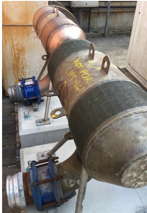
Figure 3. Test 12-inch diameter cylindrical wedgewire screens (CWWSs) used during the study in the Piscataqua River to test and compare the performance of 0.8-mm slot width (top CWWS) and 3.0-mm slot width (bottom CWWS) at reducing entrainment at Schiller Station.
