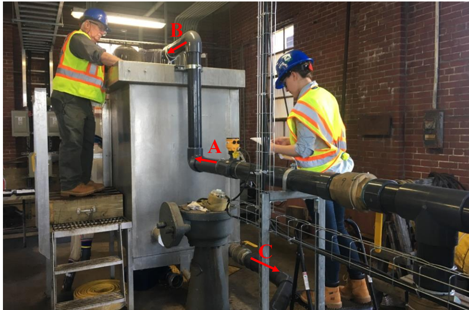
Figure 6. Entrainment sampler showing flow patterns through the tank. A: Intake flow to sampling tank. B: Flow path for water during entrainment sampling (top fill filters down through conical net and sample is collected in cod end). C: Drain line connected to tank stand pipe.
