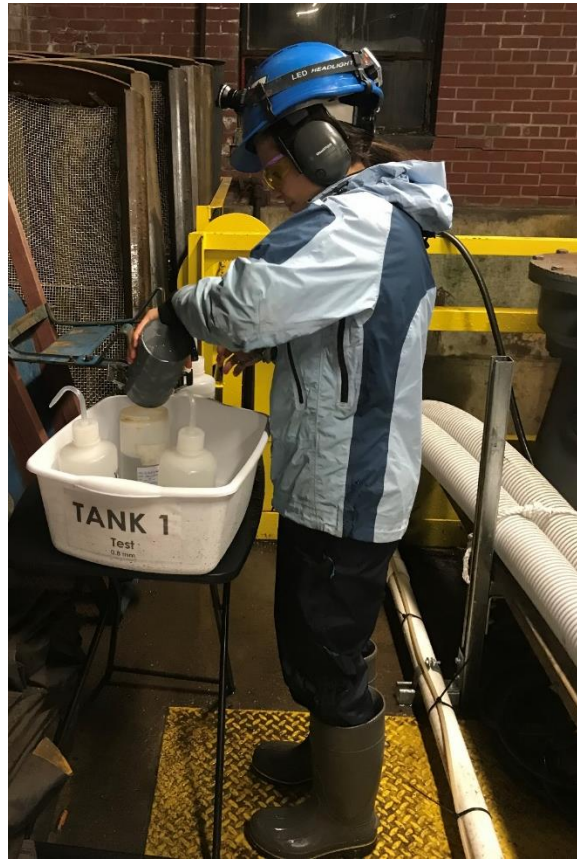
Figure 8. A 0.8-mm CWWS entrainment sample being rinsed with filtered seawater from a sampling cod end into a labeled sample jar.
