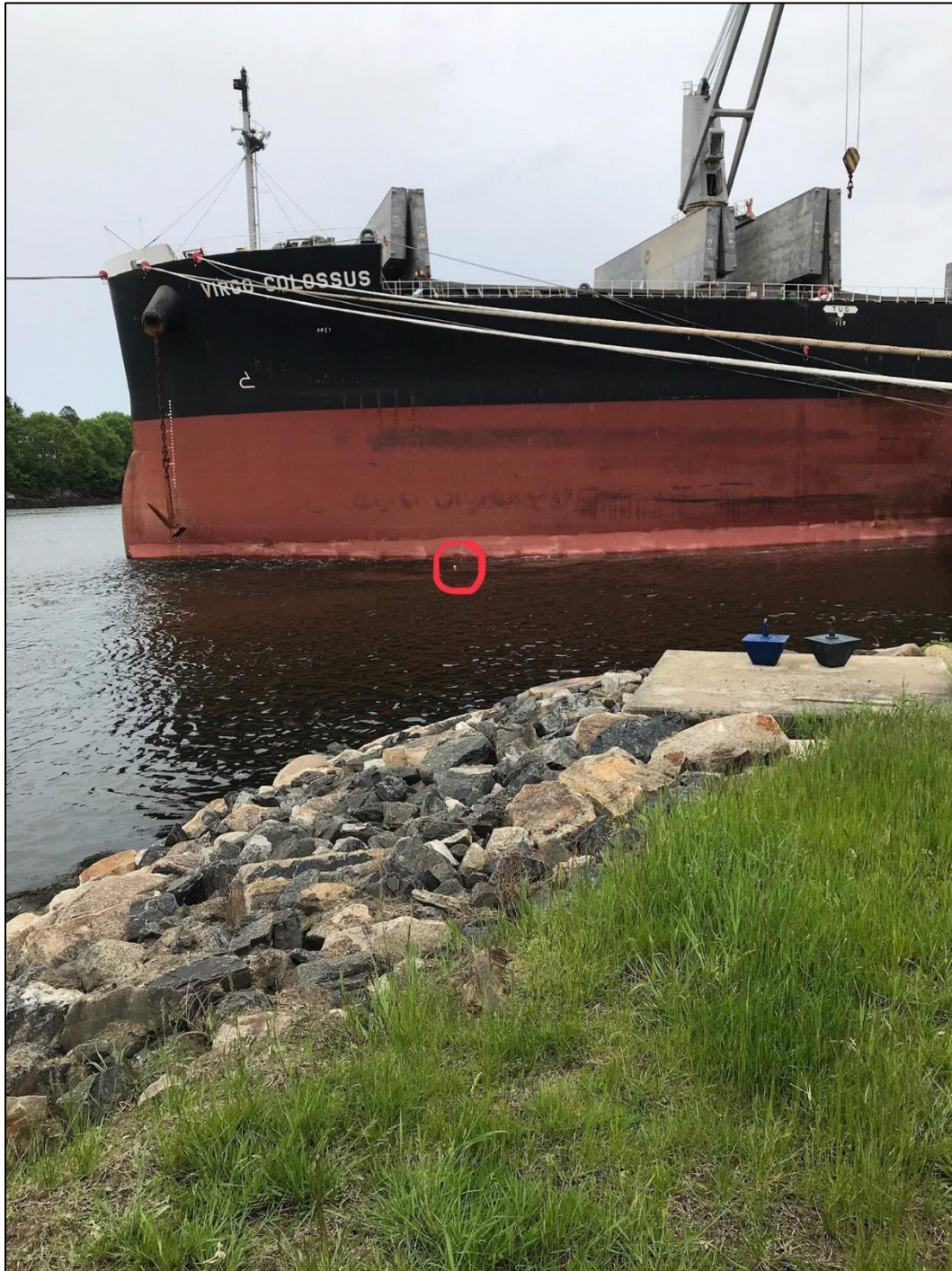
Figure C–8. Photo of the coal ship Virgo Colossus docked at Schiller Station from 25-29 May 2019. The red circle highlights the location of a surface float marking the CWWS locations. Both ADCPs were impacted by the ship, the North ADCP more so due to deployment position relative to the ship’s hull.
