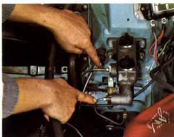
New, standard Double-Safety Brake System provides double braking protection. Two separate hydraulic systems assure braking action in emergencies. Self-Adjusting brakes, standard. Improved power brakes, optional.
