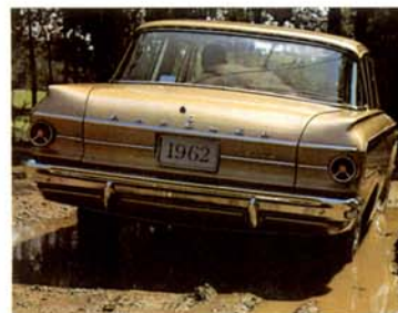
All '62 Ramblers have increased ground clearance for rough-road driving. Twin-Grip Differential is optional to give positive rear-axle traction on ice, snow or mud, or when a rear wheel slips onto a soft shoulder.
