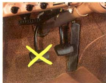
New E-Stick transmission—optional on 1962 American with standard and overdrive transmissions—gives economy and precise control of personal shifting without a clutch pedal.
