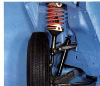
Classic and Ambassador are more stable with new Road Command front suspension featuring a new control arm and wide-track design. New, sealed lubrication. Improved power steering, optional.
