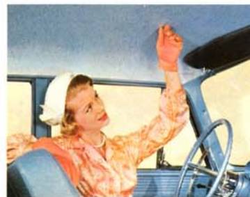
Cushioned-Acoustical Ceiling of molded fiberglass is standard on all 1962 Rambler Classic and Ambassador models. Cuts road noise 30% . . . adds to headroom. New linear texture gives smart interior appearance.
