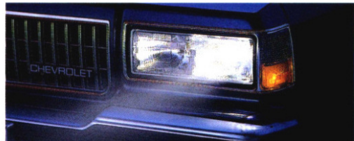
Composite-style halogen headlamps feature flush-fitting lenses and replaceable bulbs.
