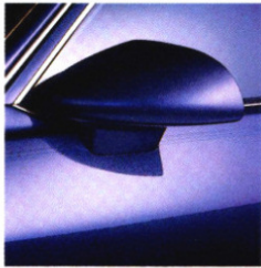
Aero-style dual sport mirrors (left-hand remote, right-hand manual).
