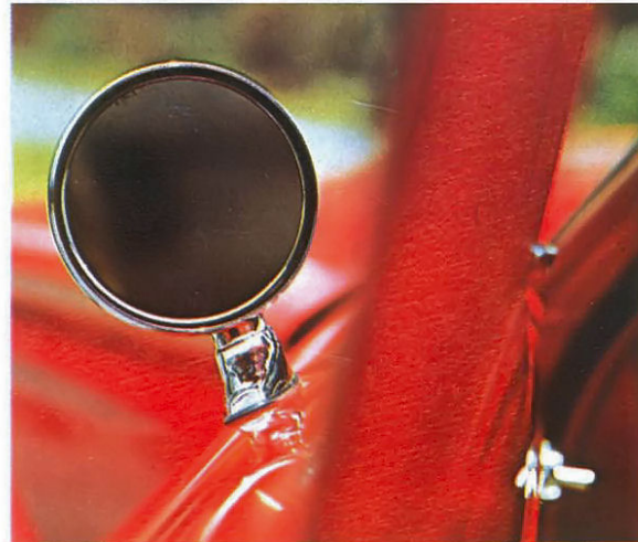
Driver can conveniently adjust mirror angle for best vision with this remote-control mirror. Control lever is located on the inside of the driver's door panel.
