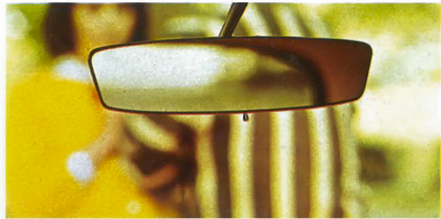
Convenient day/night mirror allows you to "turn off" annoying headlight glare from behind during nighttime driving.
