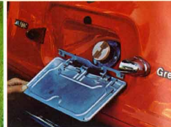
Center-fill fuel tank
