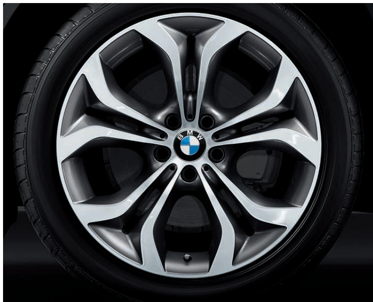
Y Spoke (Style 336) 20 x 10.0 front, 20 x 11.0 rear light alloy wheels with 275/40 front and 315/35 rear run-flat 1 performance tires. 2
