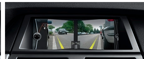
Side-view Cameras offer visual assistance when side visibility is limited, such as when exiting a parking garage or parking space. One camera is located on each front fender, just ahead of the wheel arches.
