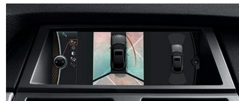
Rear-view Camera with Top View is automatically activated by shifting into reverse gear, or manually by pressing the Parking Assist button. The color Display shows a real camera image that may include "static" and "track" lines to help you when backing up or parallel parking.
