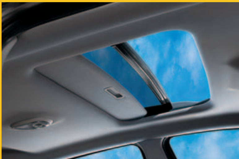
The power tilt-sliding sunroof includes an express-open feature and a wind deflector. Available on LT models.
