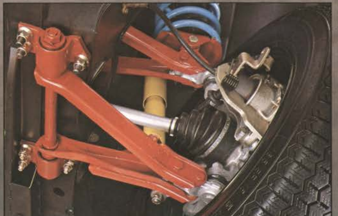
The front-wheel suspension with double wishbones is light but strong. The springs pivot and, therefore, always perform at full capacity, without tending to bend. Together with the long spring travel, this provides superb roadholding, even on irregular surfaces.
