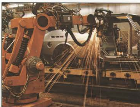
Advanced automatic welding contributes significantly to the overall sturdiness of the body.
