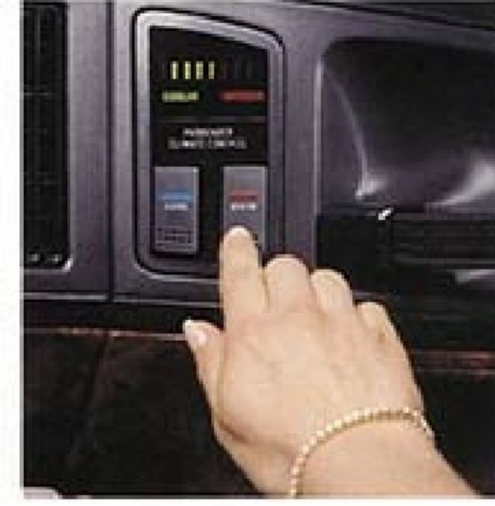
With the standard dual-zone ComforTemp automatic climate control system, the front seat passenger can determine his or her own temperature setting.
