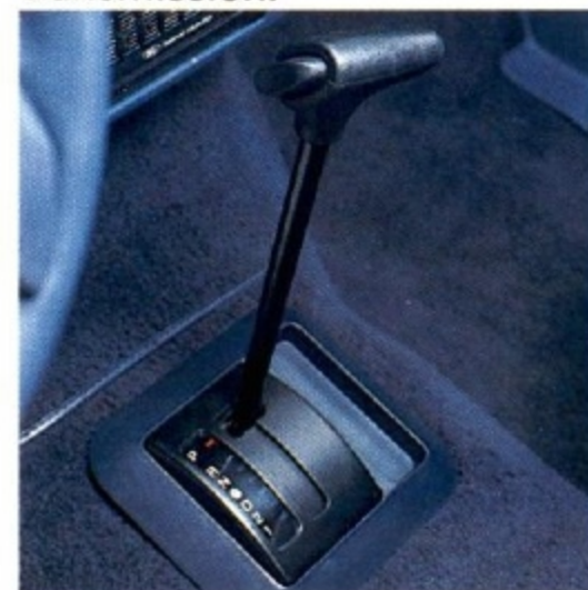
Automatic Overdrive transmission.
