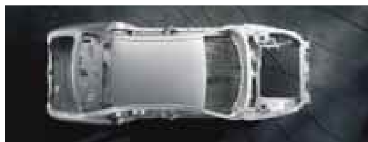
Malibu's very strong body structure includes a protective steel safety cage that surrounds the passenger compartment.
