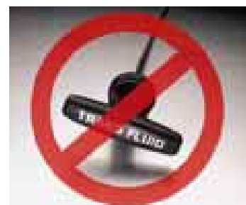
The standard electronically-controlled 4-speed automatic transmission is filled with Dexron® III transmission fluid, which never needs replacing, under normal conditions.
