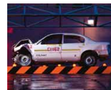
Crush zones at the front and rear are designed to absorb crash energy, in order to reduce the impact on the passenger compartment.
