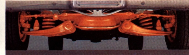
2-WD girder-beam independent front suspension
