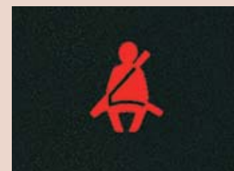
Driver seatbelt warning light in the Ambiente, Elegance, vRS and Laurin & Klement.
