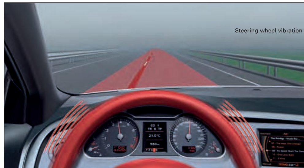
Audi lane assist – steering wheel vibration
