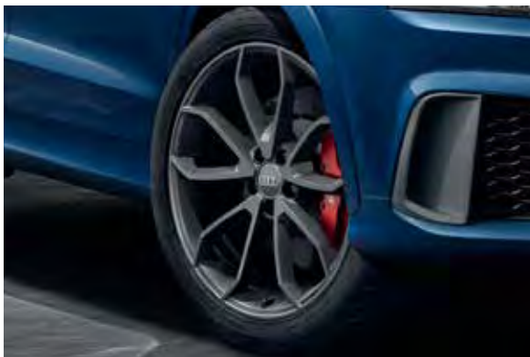
20" x 8.5J '5-twin-spoke-V' design titanium alloy wheels and Red brake calipers
