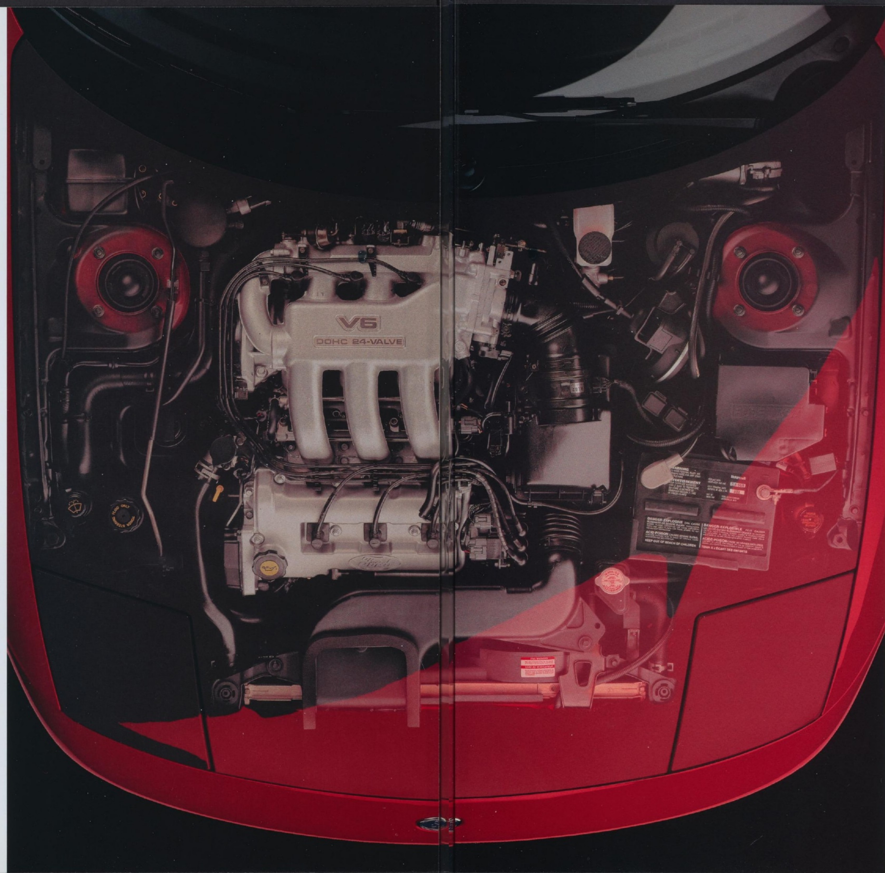
Computer-controlled, multi-port electronic fuel injection provides precise fuel metering for efficiency and smooth operation.
