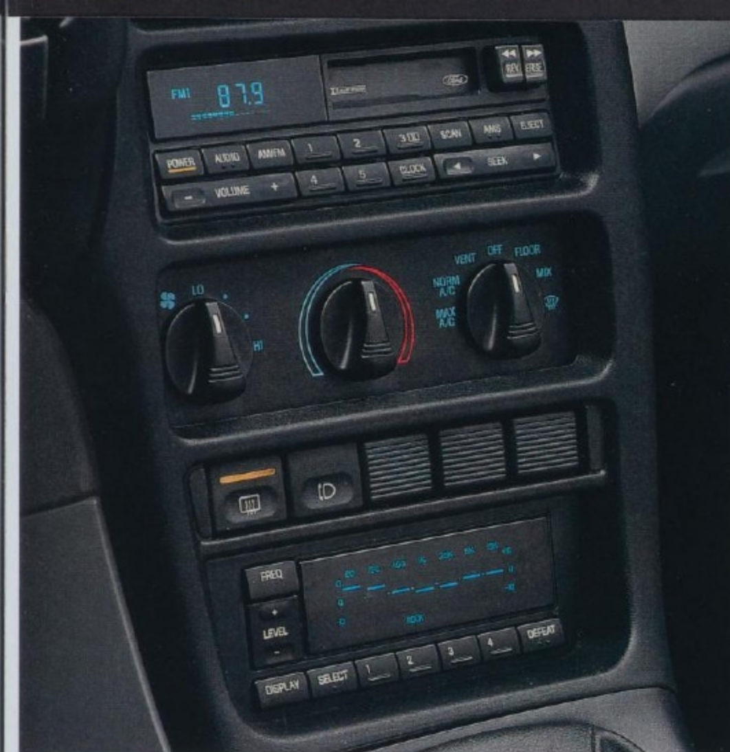
On the center panel console are heating/cooling, stereo system and other controls. This console (shown on pages 8-9) is angled toward the driver, an important ergonomic design feature.
