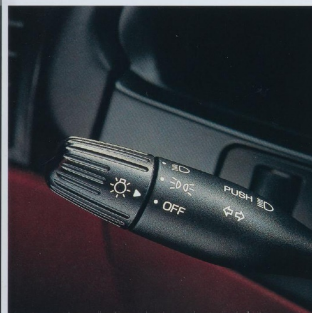
Several important operating controls (headlamps, turn signals, windshield wipers/washer) are located within easy reach on two steering column-mounted levers.
