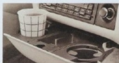
Cup holders slide out from lower center of dash to provide a secure place for beverages.
