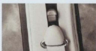
Adjustable D-rings for the driver and right front passenger improve shoulder belt comfort.
