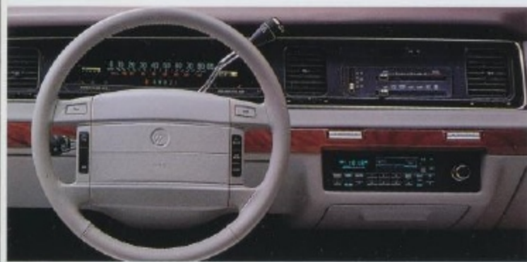
The standard analog instruments above can be replaced by an optional electronic cluster included as part of the electronic group available in LS models.
