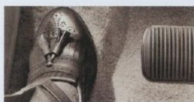
A resting place for the driver's left foot eases fatigue on long trips.
