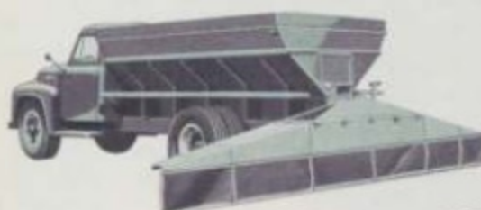
LIME SPREADER 144-, 156-, 175-in. wbs.
