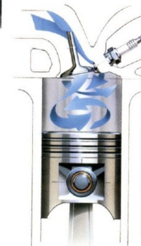
Below: Precise, efficient fuel delivery is provided to the high-swirl combustion chambers by Tempo's sequential electronic multiple-port fuel injection system.
