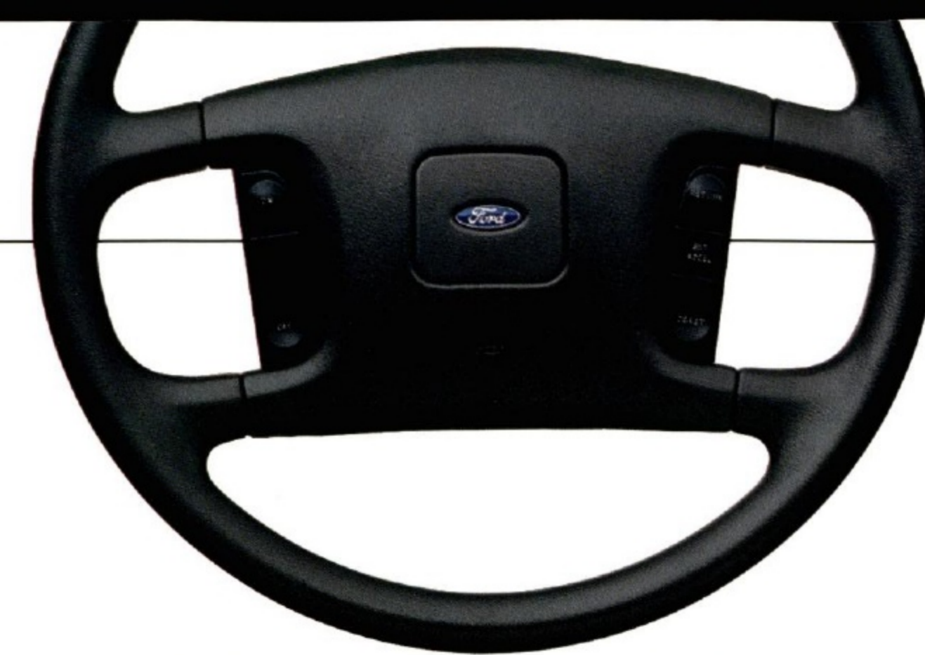
Optional speed controls are located within easy reach on the steering wheel.
