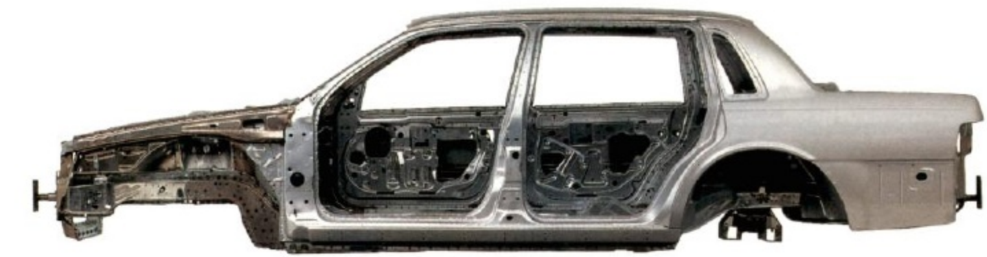
Continental's unibody structure is designed with front and rear sections, called "crumple zones," that progressively absorb much of the kinetic energy of a severe impact before it reaches the passenger compartment.
