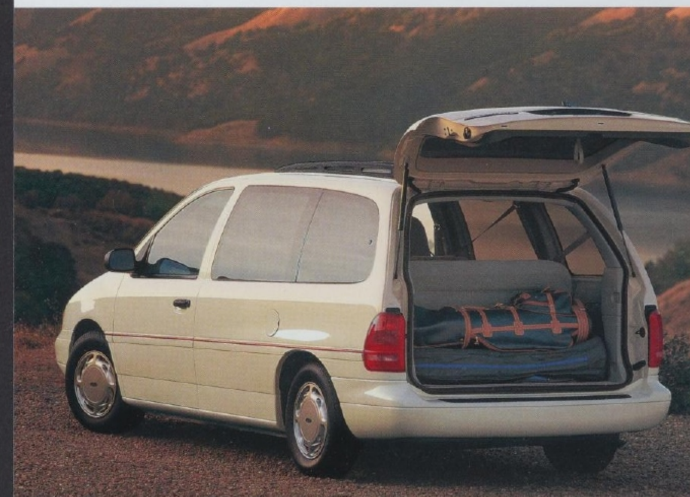
Windstar's rear liftgate opens wide for access to the generous 144 cubic foot cargo area (with the rear bench seats removed). The latch is on the side of the liftgate so it doesn't interfere with the loading or unloading of cargo.
