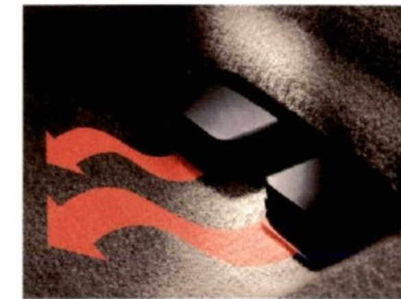
▲ Heat is distributed through vents on the instrument panel and also through rear seat area ducts.
