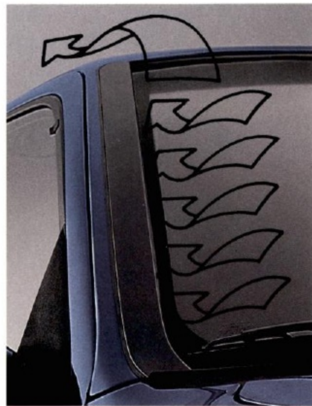
◀ Contour's windshield water management system: The cowl (between the hood and the windshield) is designed to remove rain water pushed down by the wipers. And catchers in the front pillars help keep water off the side windows and mirrors.
