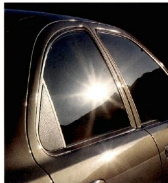
▶ Standard solar-tinted glass helps reduce heat build-up, especially when you're parked, and facilitates faster cooling when the air conditioner is turned on. Its shielding properties also help protect the surfaces of the interior from sun fading.
